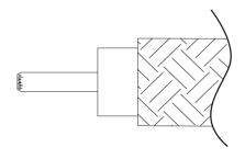
4. Chamfer the end of the centre conductor as shown.
